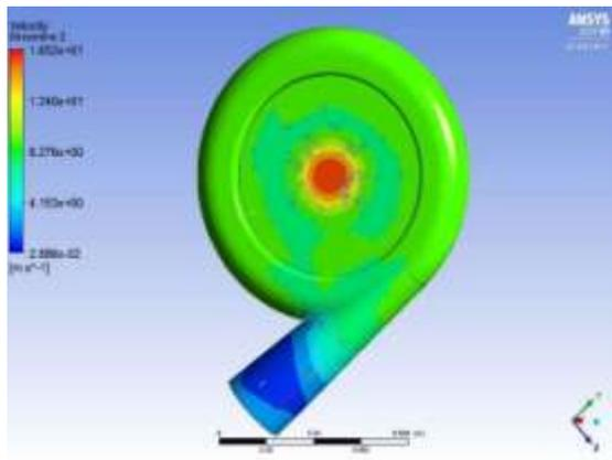
Velocity Plot for 35° inclination of the vane
